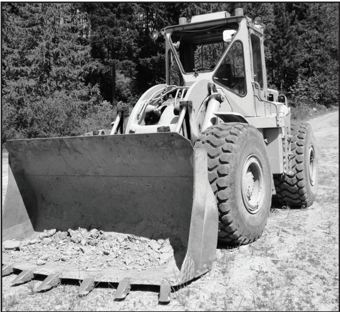
Loader with broken windshield, lights and other damage.
